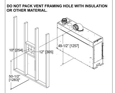
\*Shows center of vent framing hole for top venting. The center of the hole is one 1" (25mm) above the center of the horizontal vent pipe.
