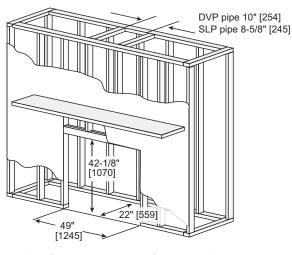
Adjust framing dimensions for interior chase sheathing (such as sheetrock)
